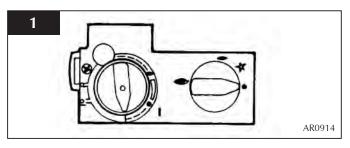
$\bullet$  Ensure that the left-hand control knob is pointing to off (  $\bullet).$
